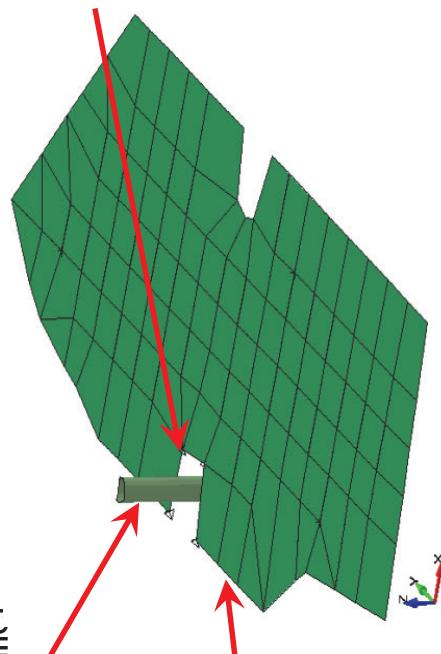
Previously a node set must be defined along the blank edge in the area of expected contact with the gage pin.
