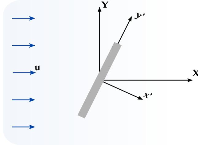
**Figure 7-6.** Anisotropic porous media vectors definition (PMMTYPE = 4, 5, 6, and 7). The vectors  $\mathbf{X}$  and  $\mathbf{Y}$  are the global axes;  $\mathbf{x}'$  and  $\mathbf{y}'$  define the system for the primed coordinate  $(x', y', z')$ .
