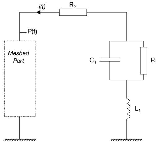
Figure 7-1. Windkessel circuit
