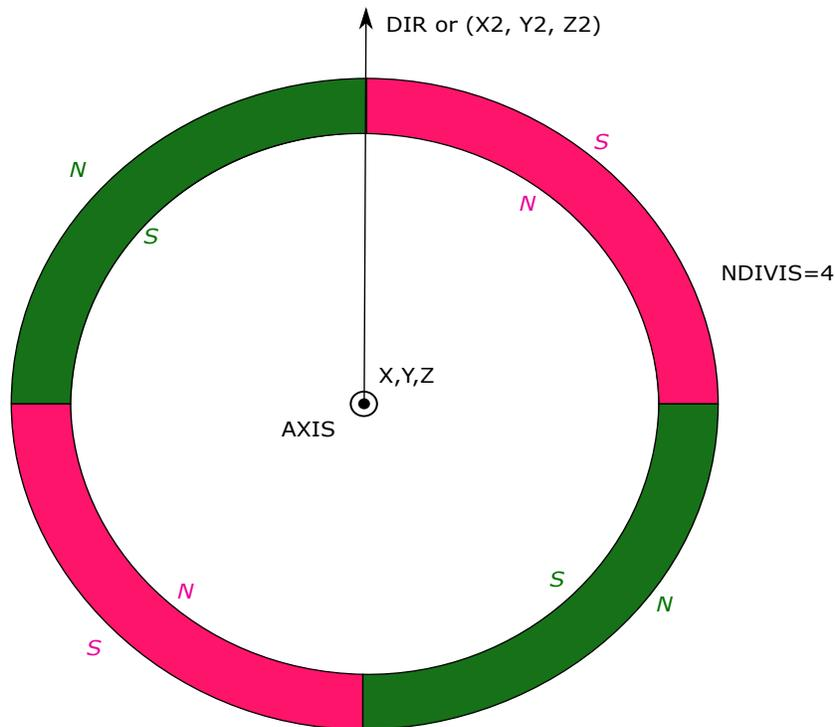
**Figure 6-4.** Example of Magnetic Gear (MTYPE = 5 or 6)
