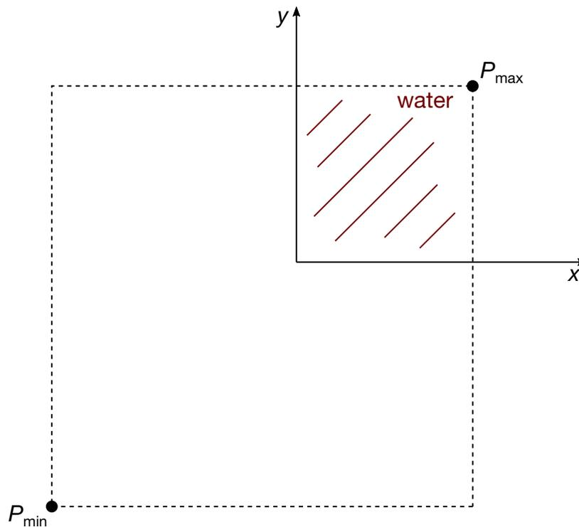
**Figure 7-5.** 2D Dam breaking example with initial levelset surface defined using  $STYPE = 2$ .  $P_{min}$  is defined sufficiently far away from the fluid surface boundaries.
