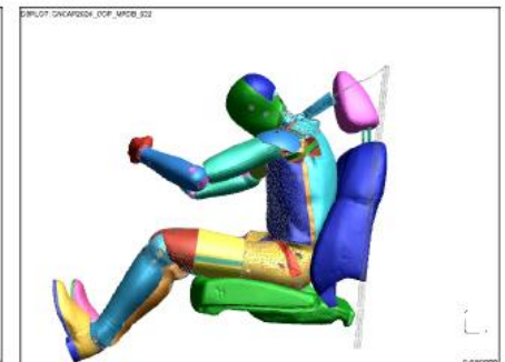
Dummy, Seatbelt and Seat only
